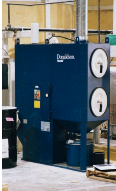
DFO on Paint & Pigment 1,200 cfm (2,038 m 3 /h)
