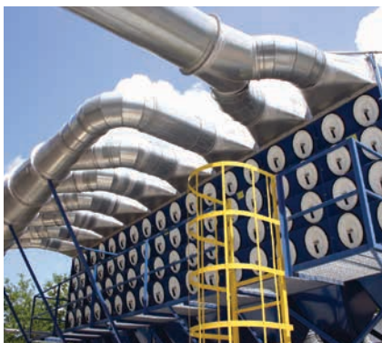
DFO on Sawdust 57,500 cfm (97,692 m 3 /h)
